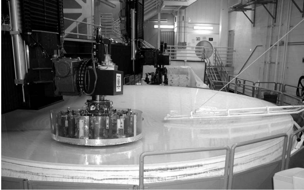
Figure 2. Second 8.4 m LBT primary mirror on the Mirror Lab's new polishing machine. Loose-abrasive grinding is being performed with a 1.2 m diameter stressed lap. A second spindle, not yet implemented, can drive an identical stressed lap or a smaller tool.
