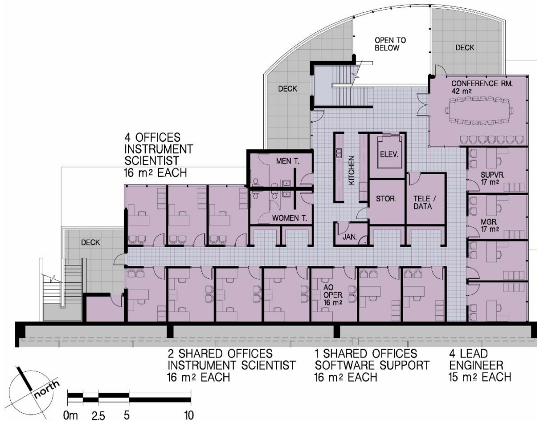
Figure 15-10. Facility Building second level.
