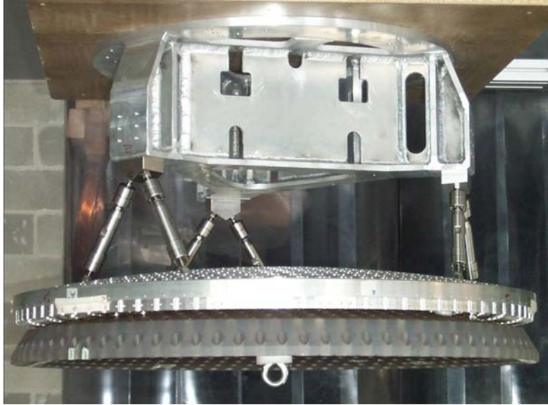
Figure 11-6. LBT reference body and actuator mounting plate with fixed hexapod support. This photo taken in the lab has been rotated 180° to show the secondary as if the telescope were zenith pointing.
