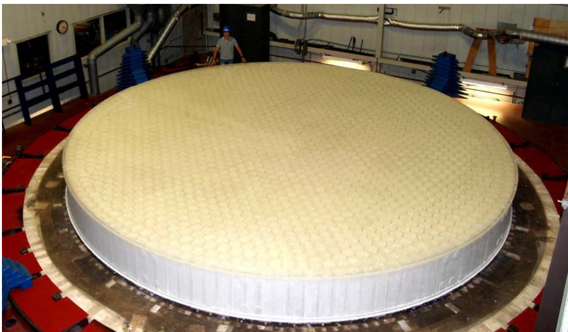
Figure 2-3. The first 8.4 m off-axis primary mirror blank for GMT in the Steward Observatory Mirror Laboratory.
