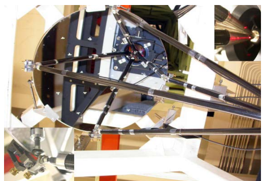
Figure 5. The CGH used 10 total patterns, used for alignment in addition to wavefront correction. The different patterns provide reference for aligning the CGH to the interferometer, aligning the 50 cm mirror, and positioning the 1.7-m mirror. The spherical mirror position was determined using four tooling balls. The lateral position of each ball was defined by light from the CGH and the axial position defined using mechanical metering rods as shown.
