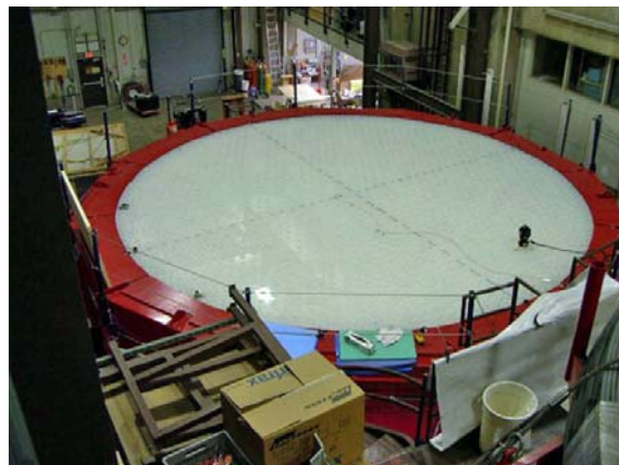
The back surface of the first GMT mirror is now being prepared prior to polishing the front surface.
